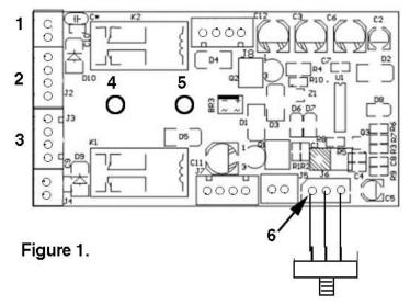
The enclosed reverse board is designed for AC current operation. This board is designed for the use with DC motors (the board will convert the AC track power to DC current).
