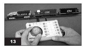
NOTE: IF YOU CHOOSE TO ARRANGE YOUR CONSIST SO THAT ONE ENGINE IS RUNNING FORWARDS AND THE OTHER IN REVERSE, ONE ENGINE MUST BE PROGRAMMED TO OPERATE IN REVERSE AS DESCRIBED IN THE "PROGRAMMING FORWARD AND REVERSE OPERATION" SECTION.
