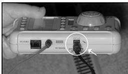
When using a track system other than *E-Z Track*\*, you will need to cut the square plug off of the *E-Z Track*\* Power Wire. Use a wire stripper to expose bare wire at the cut point, and plug the other end into the *E-Z Command*\* *Plus* Control Center. Next, attach the bare ends of the power wire to the points where you previously supplied power from your DC controller to your layout.
