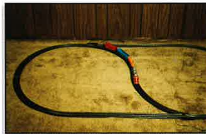
DO NOT arrange the track in a reverse loop like this. Yes, it will allow the train to turn around, but a short circuit will result unless some special insulated rail joiners and reversing electrical switch is used. Model railroad
